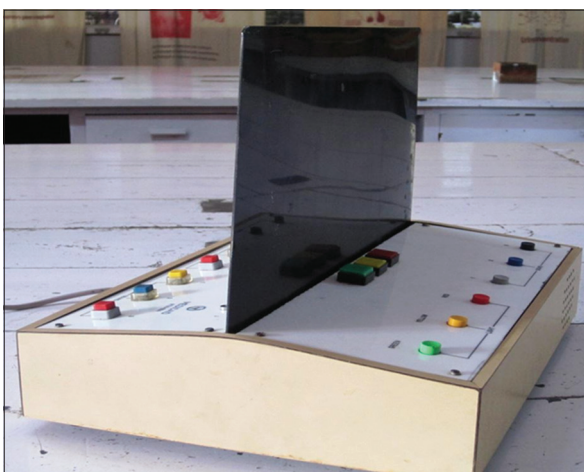
Figure 3: Reaction time apparatus showing subject component
