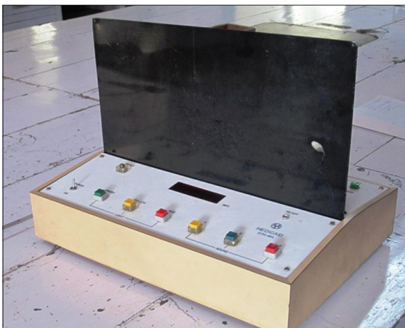
Figure 2: Reaction time apparatus showing examiners component
